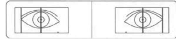
Fig.7b (The left and right pointers coincide with the reflecting bright dots)
